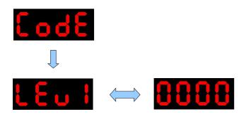
Select this option if you want to password protect the menu system. Select "NONE" for no menu protection or select "LEV1" for menu level 1 password protection. If "LEV1" is selected then the user can enter a 4 digit password. If a password has been set and "LEV1" has been selected then the large display will display "CODE" when entering the menu system. If the code is correct then it will allow the user into the menu system otherwise it will return to the normal display mode.
